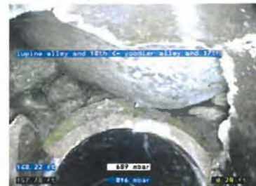
▲ Huge Hole and Boulder in Sewer Pipe
