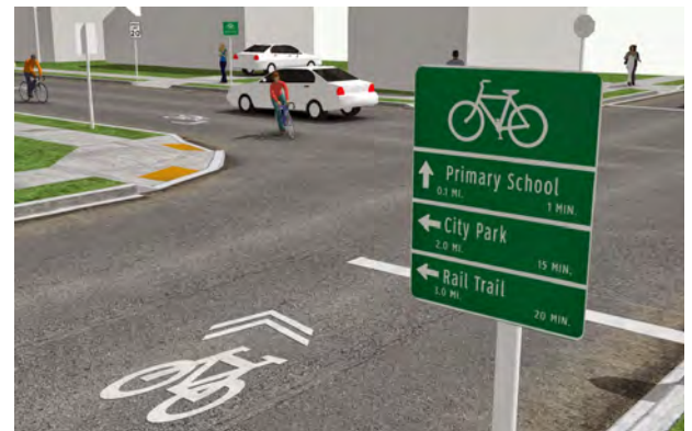
A BIKE DECISION SIGN CAN PROVIDE DESTINATIONS AND ARROWS. DISTANCES AND TRAVEL TIMES ARE OPTIONAL, BUT RECOMMENDED. (COURTESY OF NACTO)
