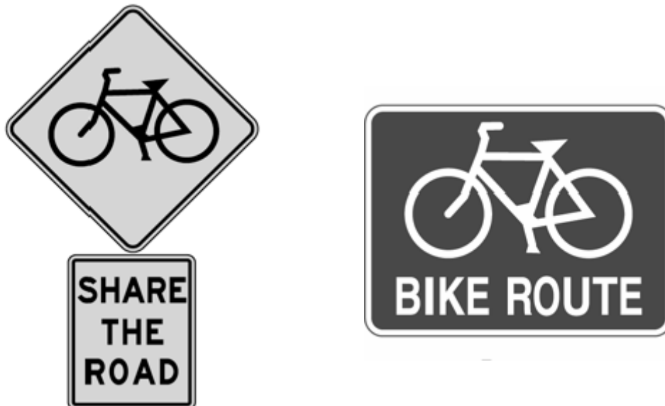
Figure B3. Examples of shared roadway signs
