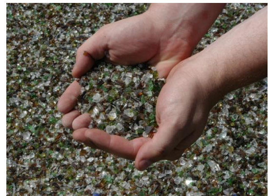
Permeable parking lot made of recycled glass in Billings
