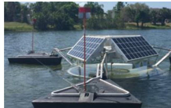
An example of a Solar Bee at a wastewater lagoon
